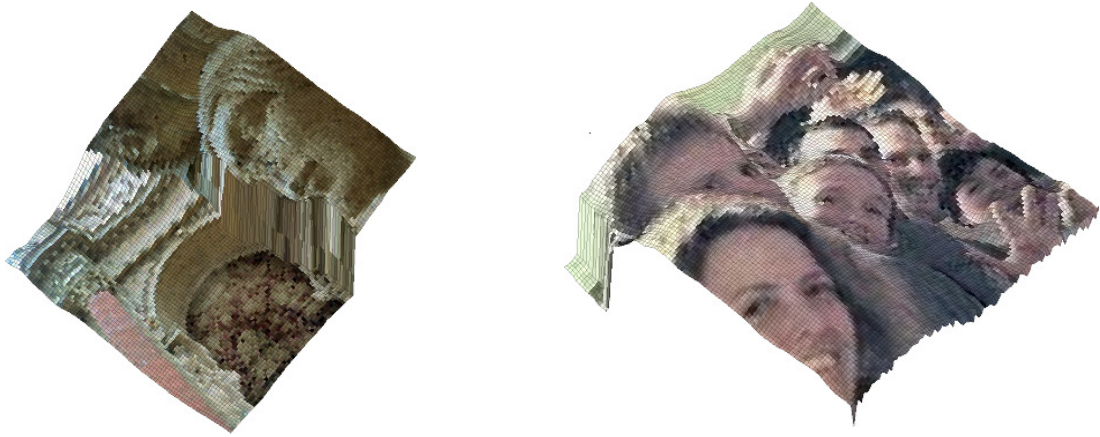
Figure 7 3D surface representation of depth with the all-in-focus image.
